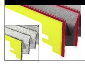
The optimum design for bellows is the heat-sealed version. The cover material and PVC guide frames are permanently joined. The connection of the bellows material and the guide frames ensures maximum loading capacity and absolute tightness against liquids such as cooling or grinding agents.
