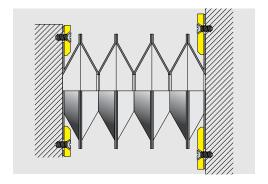
**Flange:**Different fixing devices are possible on either side.
