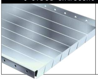
These folded bellows feature lamellas on three sides combining the advantages of telescopic steel covers with folded bellows. Thanks to this special configuration of lamellas, the bellows are protected on each side, especially against hot, sharp chips or mechanical strain. Due to an ideal ratio between the extended and the compressed length and compact dimensions – the lamella has no overhang – this type of bellows is perfectly suited to limited space applications.
