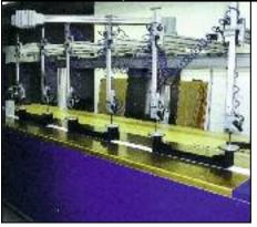
High-frequency welding of bellows is also available on special request. Patented by Hennig in Germany, it provides a homogeneous connection of bellows covers and guide frames. This method is especially well suited to the manufacture of apron covers up to 3 meters high.
